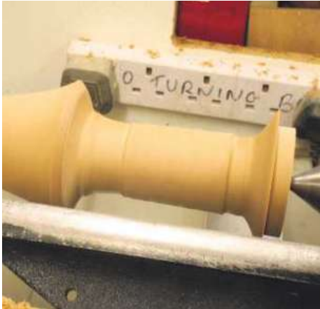
▲ Pic.19 Mount the base back onto the lathe. The lid is put on and the tailstock is brought up for support. It's imperative that your centres line up at this stage as you are going thin
